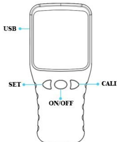
SET button: the machine requires warm-up time 60 seconds to achieve the best performance; long press the button for 3 seconds to cancel the warm-up
